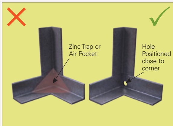
Figure 23: Inward Facing Angles – Venting Required
