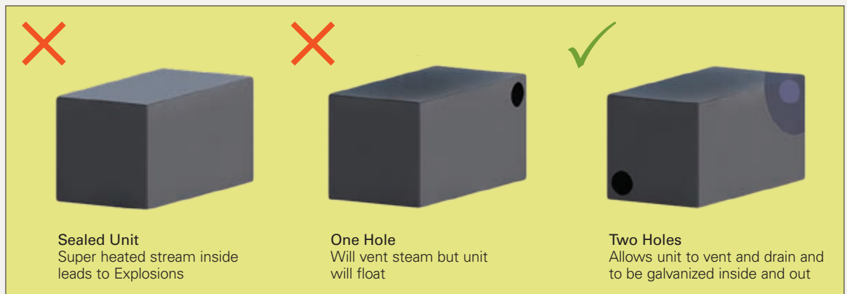
Figure 1: Purpose of Venting and Draining
