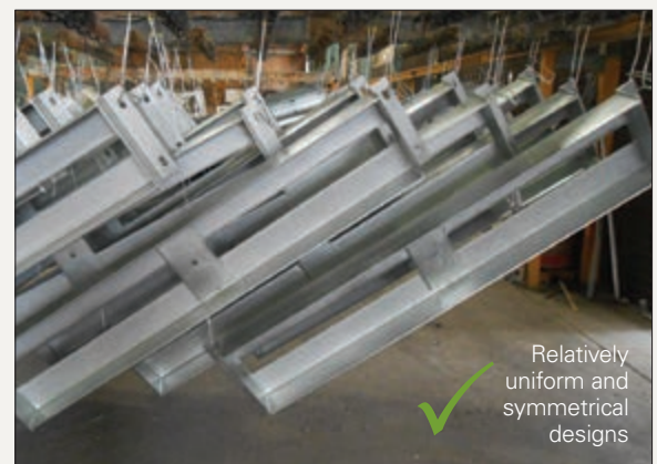
Figure 5: Avoid Distortion with Good Design
