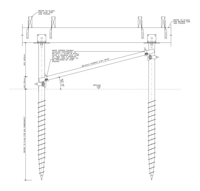
The StopDigging steel bracing system provides higher lateral support to piles to allow for high subfloor levels above ground, and design solutions for sloping sites.
