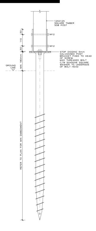
Using our SGE 125 bracket, Stop Digging Groundscrews are used as a spot footing for connection to a standard timber senton house pile (125x125). Posts are braced as normal to standard NZ3604.
