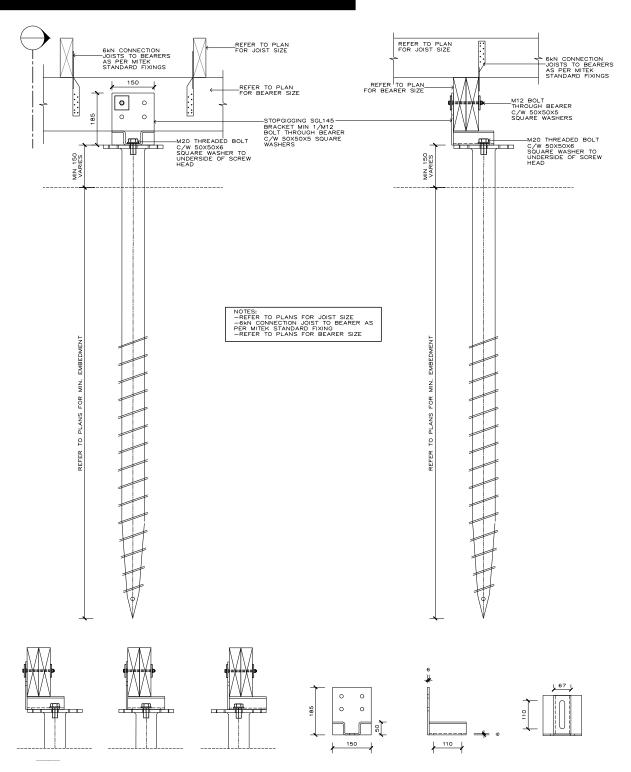
Using our SGL145 bracket, StopDigging Groundscrews are used as a cantilever pile for house and deck foundations. The SGL 145 provides both a 6kN or 12kN connection, and allows for up to 100mm of lateral tolerance for easy site alignment.
