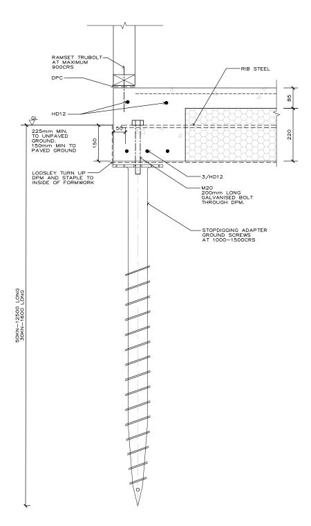
Stopdigging Groundscrews are used as an alternative to a deepened perimeter footing or cantilevered slab design in either expansive ground or ground with low bearing capacity. The ground screws extend beyond the influence of the shrink-swell zone, or low bearing capacity and support the slab edge and any point loads.
