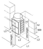
Add the dimension that exceeds the height limit (shown as "h1" through "h3" in the figures) to L1, L2, and L3 as shown in the table below.
