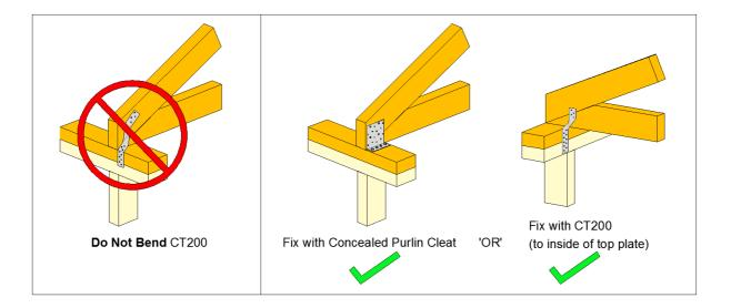
The MiTek 20/20 software doesn't identify this fixing detail arrangement and may select WIREDOGS or a CEILING TIE by default. If it does, please replace by using the table below, or by referring to the fixing report in MiTek 20/20 and the LUMBERLOK characteristic loadings brochure.
