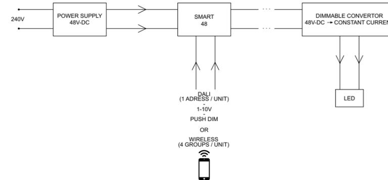
New in Lighting Bible 12 is the possibility to dim 48V luminaires or profiles, thanks to Smart 48. It collects the power from the 48V power supply and combines it with a DALI, 1-10V or Touch Dim input and sends it to the 48V converter in the luminaire. With the Dimmable Modulator 48V-DC DIM9, dimming can be done by only using 2 wires for both power and dimming. Or dimming can be done wireless, by choosing for the Wireless Dimmable Modulator 48V-DC.
