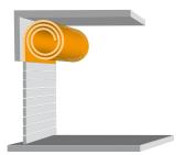
The round spiral is the standard and best solution when you have ample space above the door.
