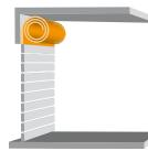
New: The EFA-SST® PS features a spiral construction that significantly reduces the space requirements in the lintel.
