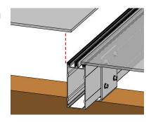
glazing bar in the bracket and attach using the stainless steel self drilling screws provided. The screw hole centres should align with the visual lines on outside wall of the glazing bar.
