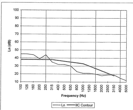
\* Due to high insulating value of specimen, background levels limit results at these frequencies.
