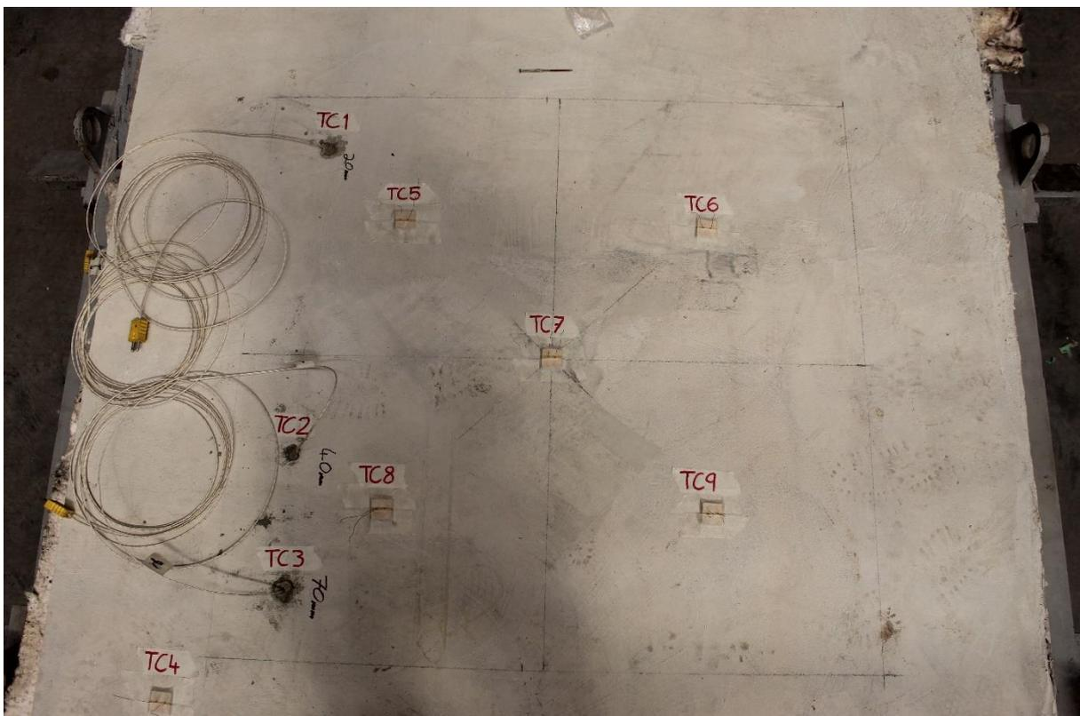
The separating element has been constructed with a 1.45m x 1.45m x 75mm concrete topping on a 900mm<sup>2</sup> bed of 150 x 25 rs h3.2 timber infills.
