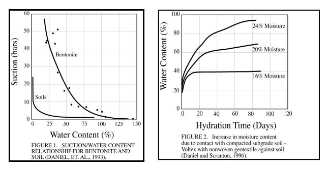
Figure 2 shows a hydration curve for Voltex<sup>®</sup> placed on soil subgrades of varying moisture contents. It can be seen that Voltex (with no water added to the system) reaches a steady-state value after a period of approximately 90 days. It is important to note that the bentonite component of Voltex can only absorb water available in close proximity to itself; in each of these cases, the overall soil moisture values did not measurably change during the test period. This
