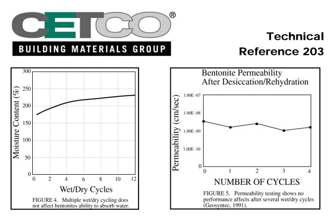
**CONCLUSION:** There is a clear and persuasive data that "wet-dry cycling" does not occur in Voltex and should not be considered a problem. Even if such cycles were to occur, Voltex has been proven to rehydrate and reseal in the presence of water.
