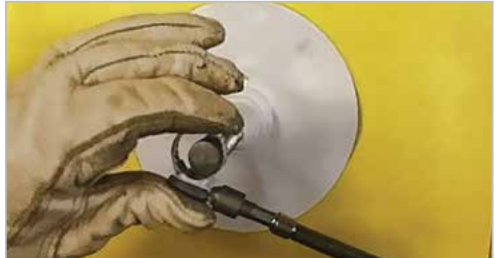
STEP 6. Hose Clamp Loosely Installed
