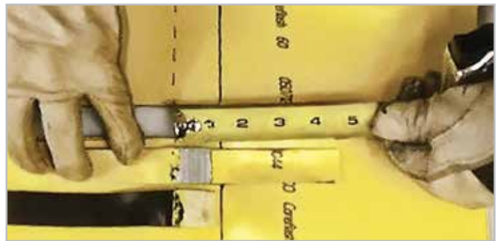
STEP 4. Weld width verification
