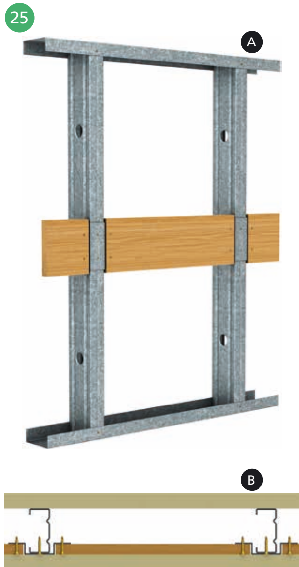
■ TIMBER NOGGINGS NOTCHED TO FIT BETWEEN STUD WEBS
