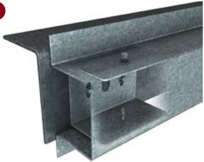
■ TOP HAT FIXED TO STEELWORK FIXINGS: CLEAT TO STEELWORK AND TOP HAT TO CLEAT WITH #12 TEK SCREWS AS SHOWN
