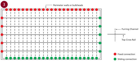
KEY-LOCK<sup>®</sup> CEILING PLAN – TYPICAL PERIMETER FIXING ARRANGEMENT
