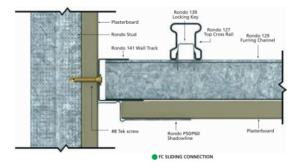
KEY-LOCK® FURRING CHANNEL FIXED AND SLIDING PERIMETER CONNECTION DETAILS
