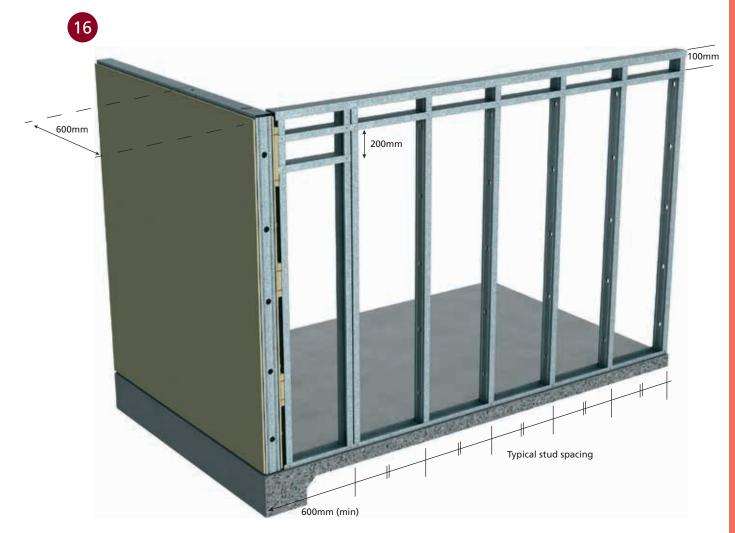
NOTE: This is a pictorial only, a midspan nogging may be required depending on wall height and lining conditions, refer to the Rondo Professional Design Manual for nogging requirements.
