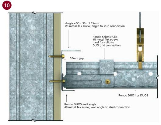
DUO GRID FIXING TO STUDWALL — FIXED CONNECTION
