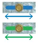
Indicates the fixing slot in the Rondo Seismic Slotted Deflection Head Track. The slot allows displacement of adjacent Wall Studs, letting them slide within the Tracks in the direction shown by the arrows. The movement occurs at the head whilst the wall framing is stabilised at the base.
