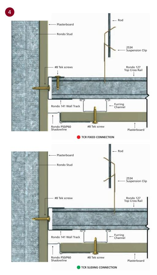
KEY-LOCK® TOP CROSS RAIL FIXED AND SLIDING PERIMETER CONNECTION DETAILS
