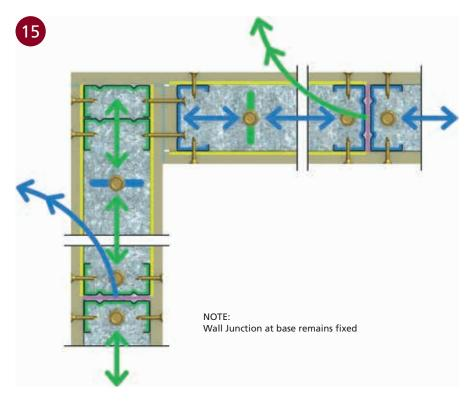
STUD WALL ARTICULATION/MOVEMENT AT CORNER JUNCTION AT HEAD
