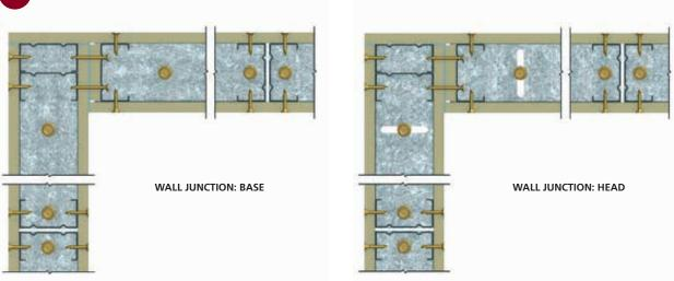
SEISMIC STUD WALL ARRANGEMENTS (STANDARD CORNER DETAILS AT THE HEAD & BASE TRACK)
