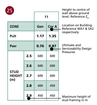
■ EXTRACT OF CONFIGURATION OF WALL STUD FRAMING TABLES, FROM PAGES 130 ON
