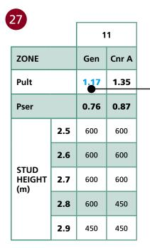
1. Check the required pressure from the Wall Stud Design Tables to identify the appropriate coloured pressure line to use in the graph. (1.17kPa Pressure in this example)
