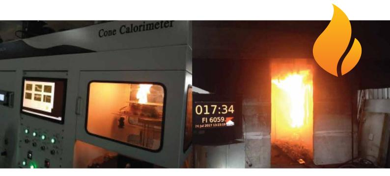
ISO 5660-1:2015 is an International Standard which specifies the heat release rate and smoke production rate. The time to ignition is also measured in this test. Total and peak heat release are the key measurement required to assess suitability of products on high rise buildings and buildings close to boundaries.
