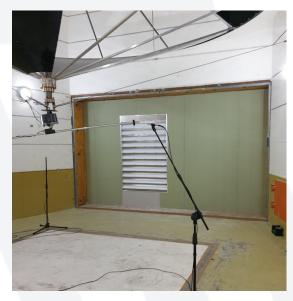
Fig. 2 - Ventüer louvres undergoing acoustic testing at Auckland University laboratory.
