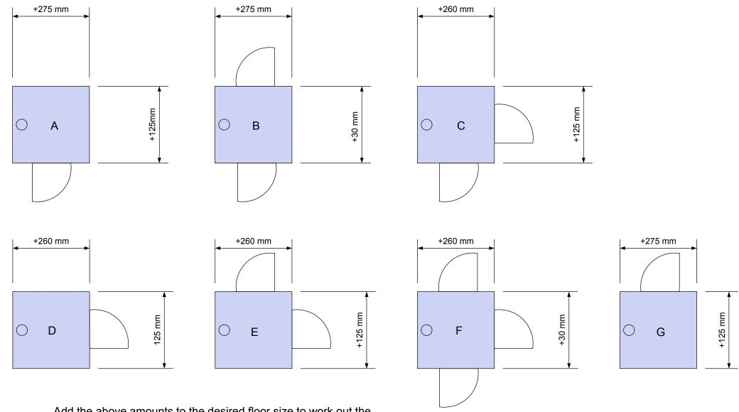
Add the above amounts to the desired floor size to work out the "finished" inside size of your lift shaft. i.e. A 1000mm floor with a door opposite the cylinder will require a 1260mm deep shaft
