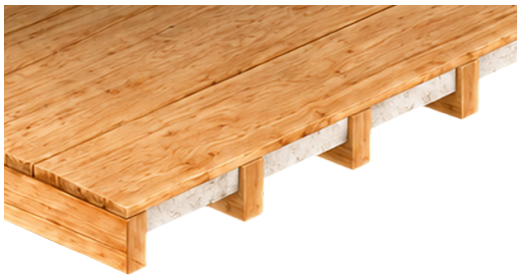
Figure 12. EcoVersal between timber joists
