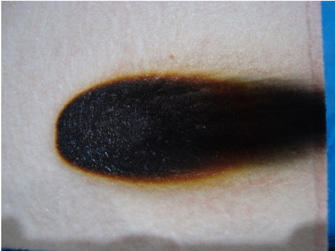
Charing of non-metallic facing material due to needle flame
