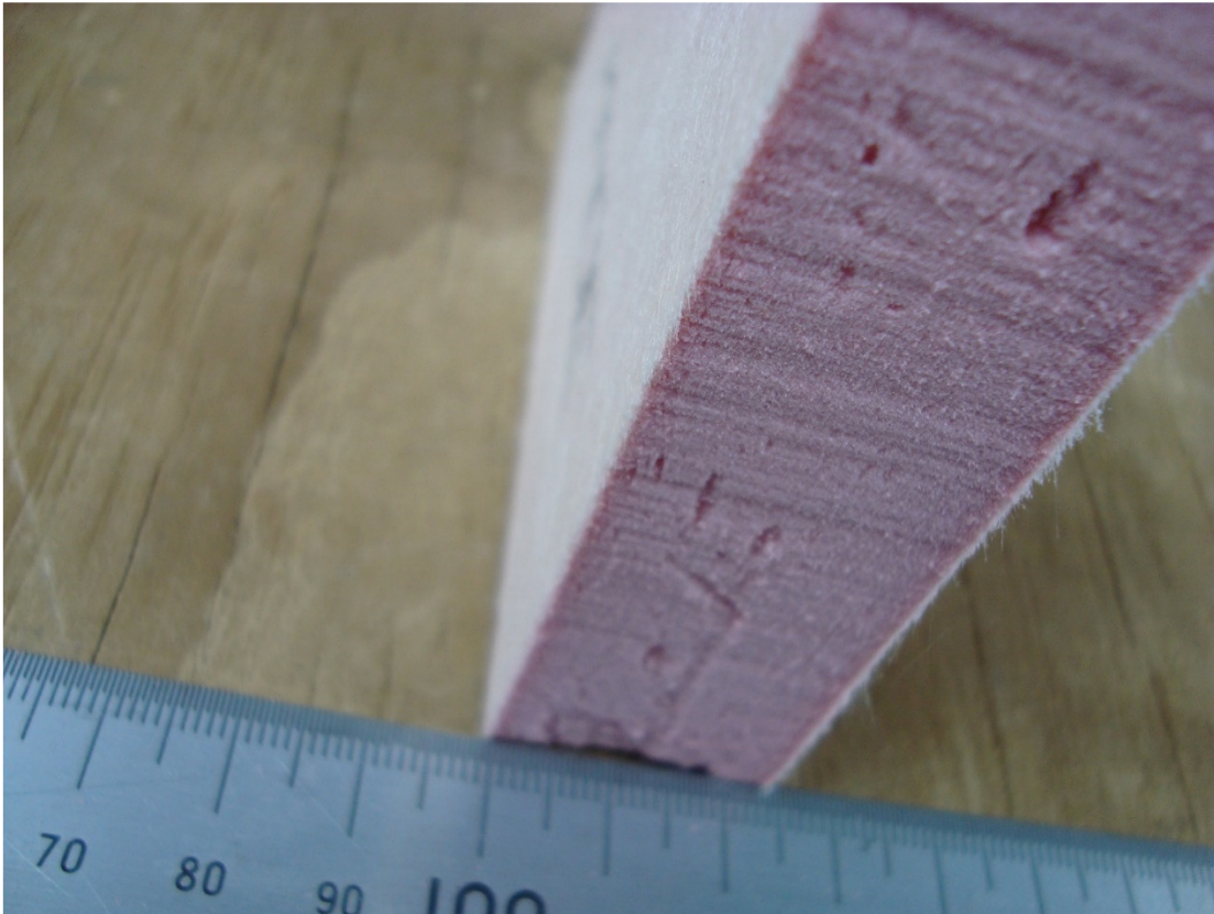
24 mm thick with non-metallic facing material
