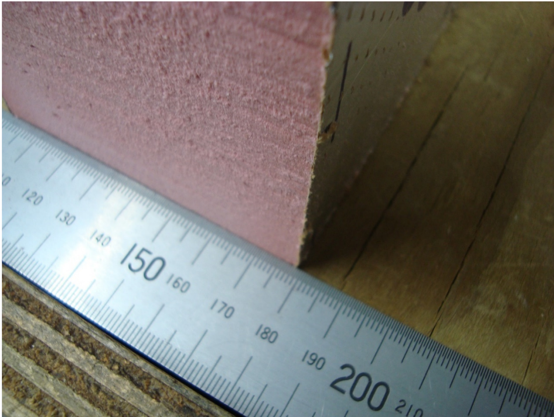
80 mm thick with metallic facing material
