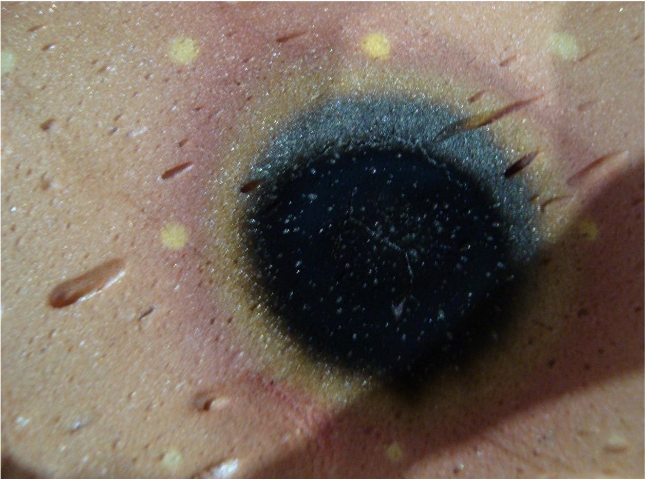
Charing of insulation material due needle flame
