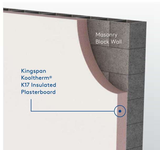
Figure 5. Kooltherm K17 Insulated Plasterboard adheres directly to masonry block wall surface.
