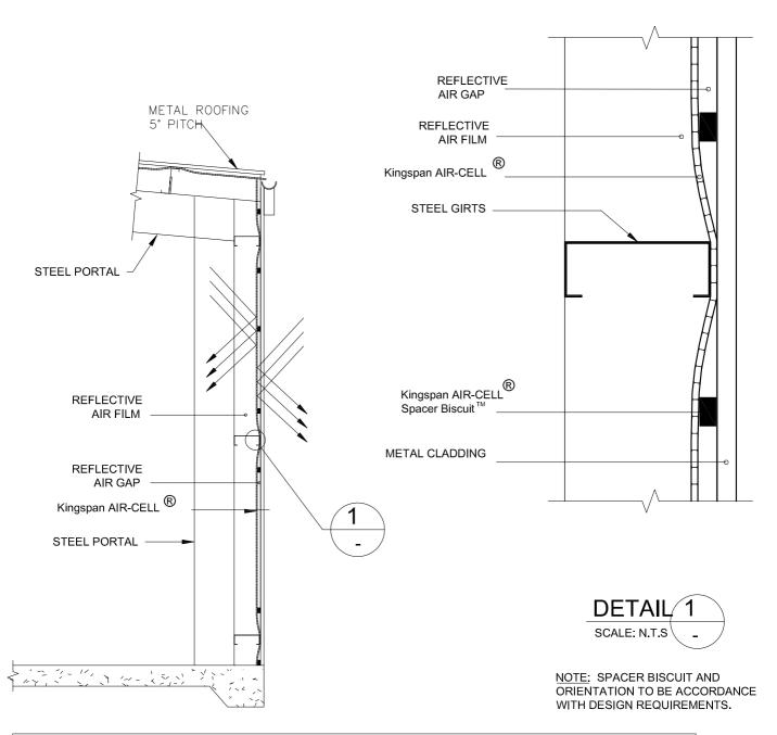
NOTE: WHERE JOINS ARE APPLICABLE, APPLY 150mm OVERLAP (TAPED OR UNTAPED) OR BUTT JOIN AND TAPE.
