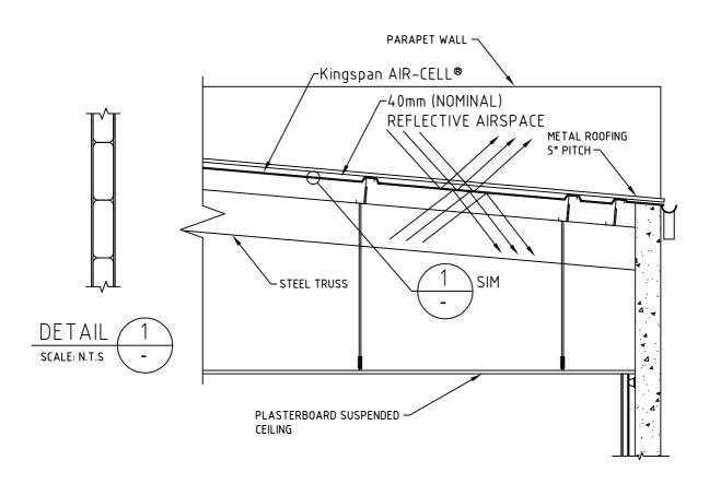
NOTE: Where a suspended ceiling is present the air space above the suspended ceiling has been assumed to be 100mm –1200mm deep. For large ceiling space the heatflow in R-value should be reduced by approximately R0.5.
