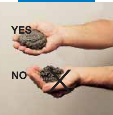
The correct consistency of Mapecem
