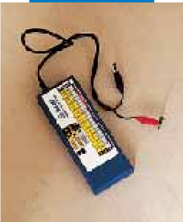
Electronic hygrometer for measuring the moisture level of a Mapecem screed
