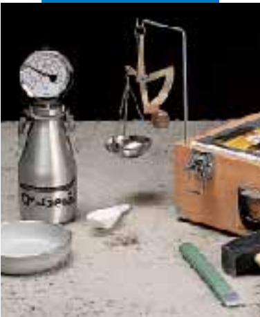
Carbide hygrometer for measuring the moisture level of a Mapecem screed
