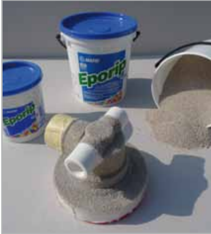
Fig. 3.7 - Applying a coat of Eporip on components for a water recirculation unit
