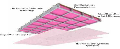
In order for GIB® systems to perform as tested, all components must be installed exactly as prescribed. Substituting mponents produces an entirely different system and may seriously compromise performance. Follow system specifications.
