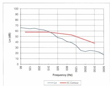
Due to high insulating value of specimen, background levels limit results at these frequencies.
