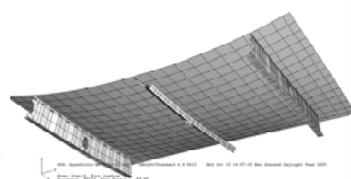
The 3D model shows a slab with a grid of reinforcement. The deflection is visualized as a downward curve across the span of the slab.
