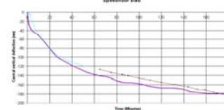
The graph shows the deflection of a Speedfloor slab over time. The y-axis is 'Deflection (mm)' ranging from 0 to 200. The x-axis is 'Time (minutes)' ranging from 0 to 120. The curve shows a rapid initial increase in deflection, followed by a slower, steady increase, reaching approximately 180 mm at 120 minutes.
