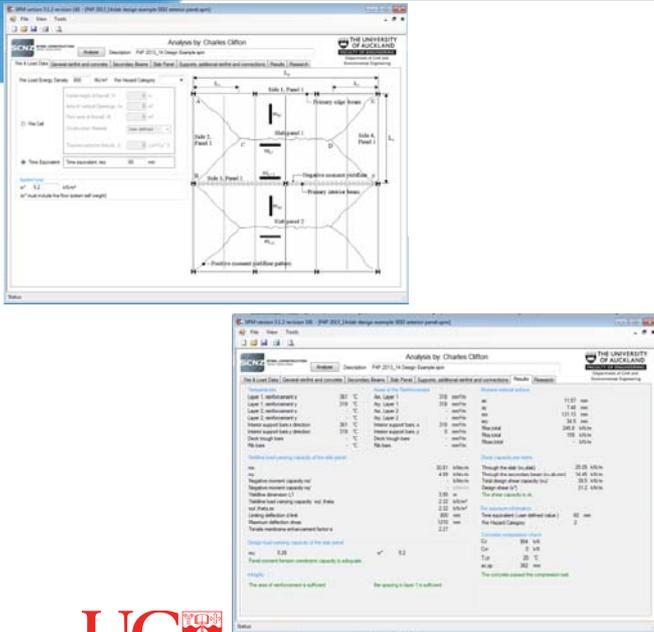
The top screenshot shows the 'Analysis' options screen with various checkboxes for 'General analysis and connections', 'Secondary Beams', 'Slab Trays', 'Supports additional walls and connections', and 'Nodes'. The bottom screenshot shows a detailed 'RESULTS' table with columns for 'Description', 'Units', and 'Value'. The table lists various parameters such as 'Slab 1 reinforcement', 'Slab 2 reinforcement', 'Deck height', and 'Deck reinforcement', along with their respective values and units.
