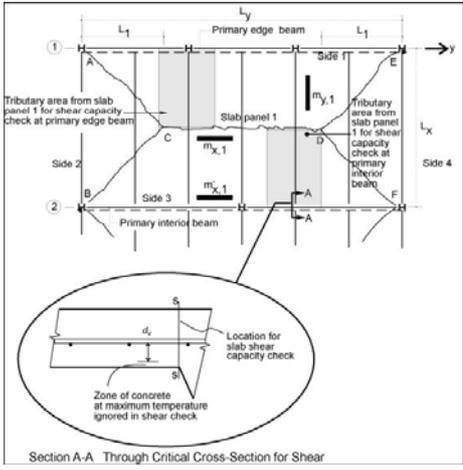
The diagram illustrates a slab panel with primary edge beams and a primary interior beam. It shows tributary areas for shear capacity checks at primary edge beams and primary interior beams. A detailed view of a secondary beam cross-section shows the location for slab shear capacity check and a zone of concrete at maximum temperature ignored in shear check.
