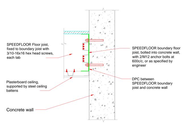
MFD 4 - SPEEDFLOOR Joist to side of Concrete or Block Wall
