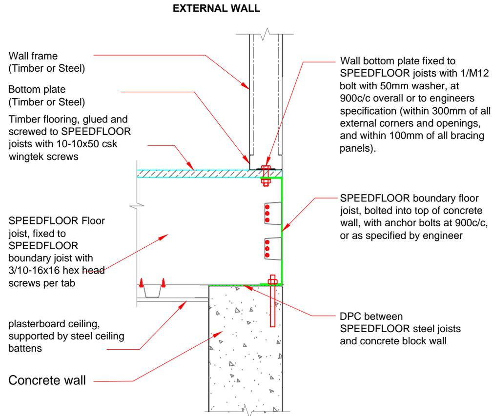
**MFD 3 - SPEEDFLOOR Joist to Concrete Wall**
