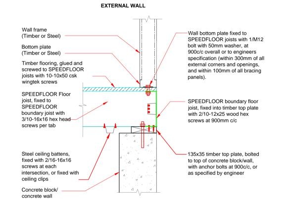
MFD 2C - SPEEDFLOOR 140 or 190 Joist to Concrete or Block Wall
