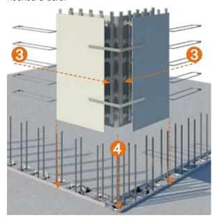
Install upper corner panels on top of lower corner panels. The panels can be installed manually or using crane depending on the panels size. Fix internal corner angle to the first upper panel to be installed as per step 2. Then plumb and brace lower panel 1 and upper panel 1 as per the standard procedure.
