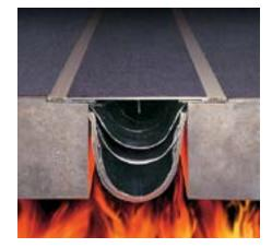
Multiple drape configurations of stainless foil and insulation utilize air pockets for additional insulation performance. Sliding frame is available for 200% lateral shear applications in floors.
