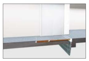
Full Closed (During Compression) During an event, the MACC system slides fully into the adjoining structure in the contraction (or compression) mode.
