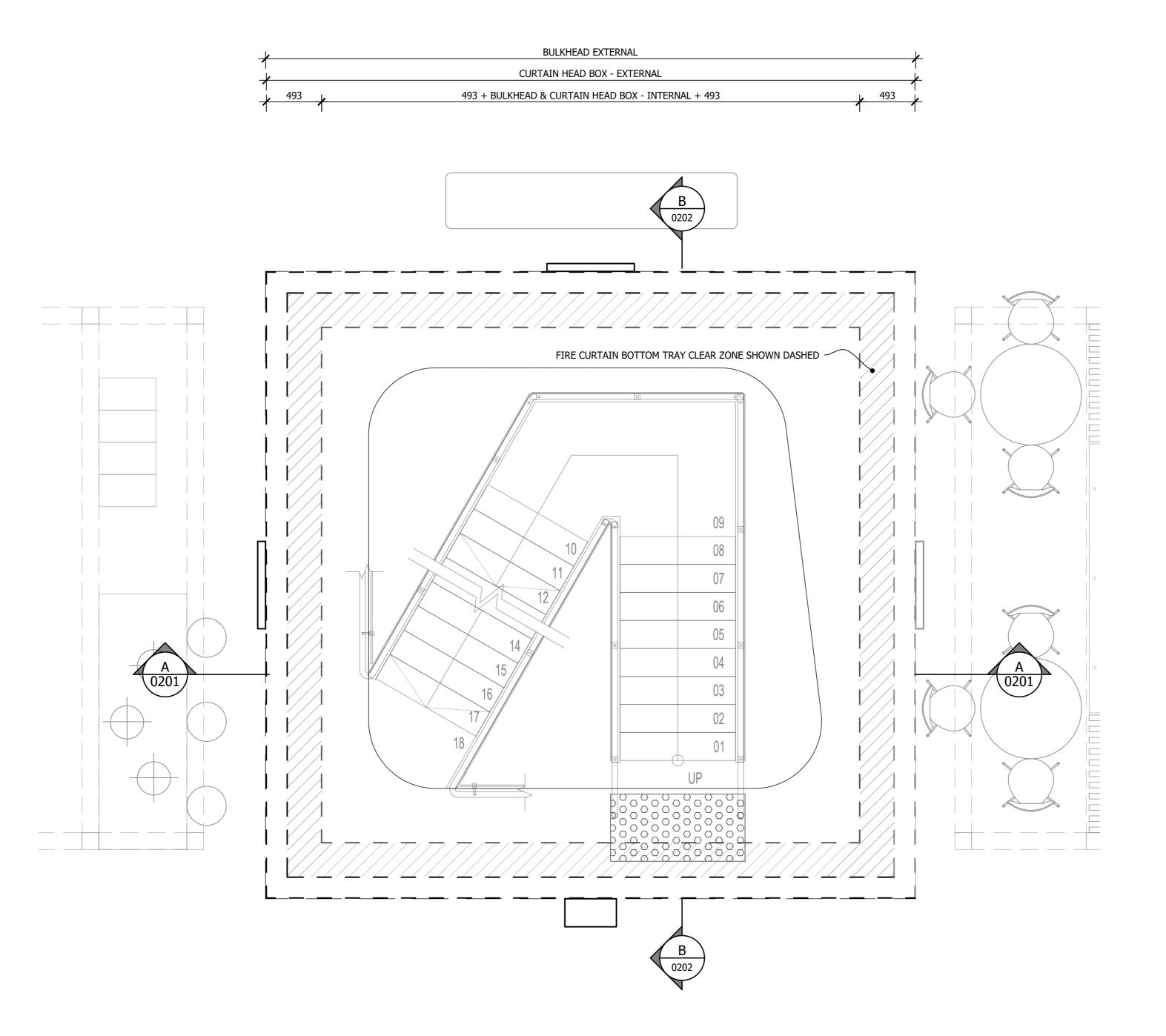
PLAN FYREHALT EVOLUTION - FIRE CURTAIN SCALE 1:25 @ A2
