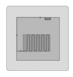
Once the underlayment/insulation has been fitted in the normal manner, remove your Warmup Foil mat from the packaging box, unroll it completely and place it in the required position on top of the underlayment/insulation. Make sure that Warmup Foil heating mats are installed with the correct orientation. The side marked "THIS SIDE UP" is facing upwards.
