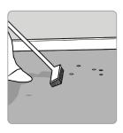
Ensure the sub floor is structurally sound. The sub floor should be clean and dry.
