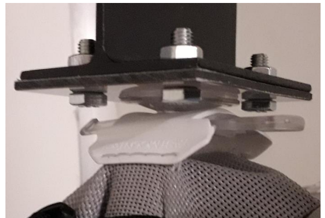
Figure 3 - Directly before separation of the female to male clips shown left and separation of adhesion layer shown right
