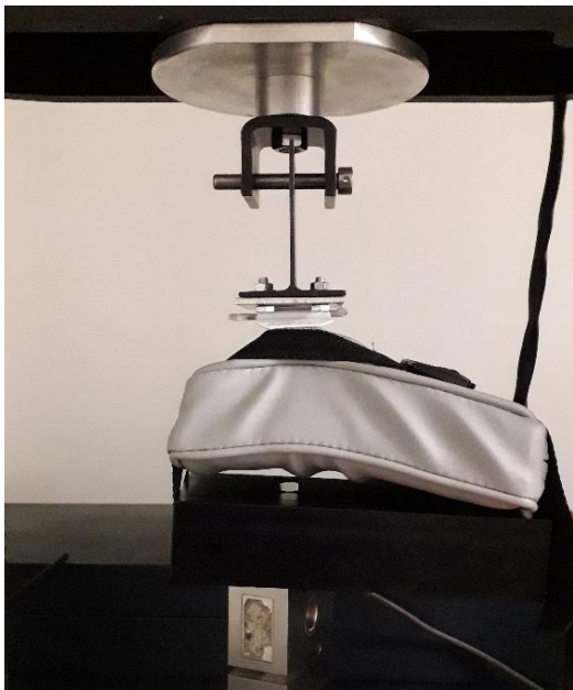
Figure 2 - TC-F6H clip under test with TC-M6 shown left and with TC-SM6 shown right.
