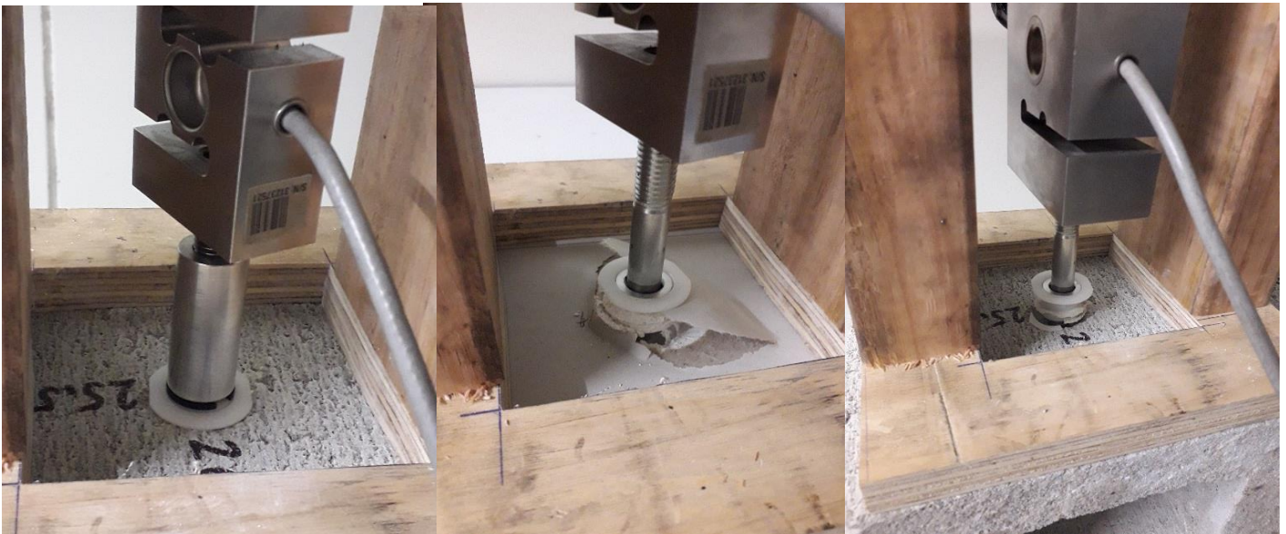
Figure 2 - Typical test setup and pull-out failures.
