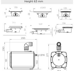
NOTE: To maintain radio signal integrity pump must be installed in same room with power cable end facing towards shower waste gully.
