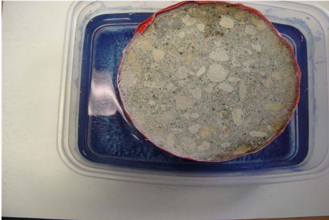
Photo (4): Lightweight concrete sample after three days from the start of the test, showing 10% saturation of the top surface area.
