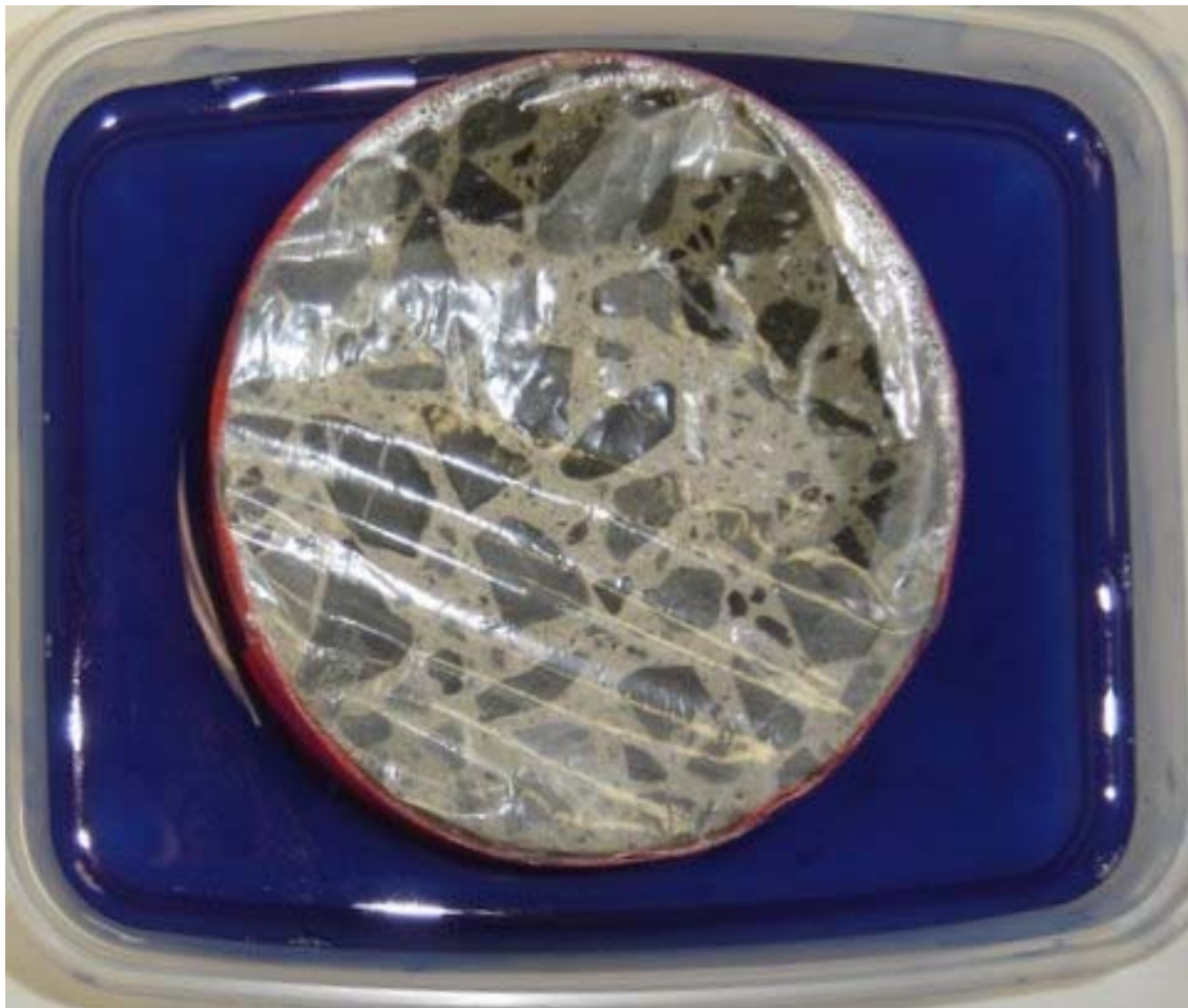
Photo (1): Normal concrete sample shows traces of water saturating 25% of the surface area after less than five hours from the start of the test.
