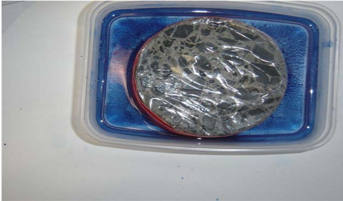
Photo (2): Normal concrete sample after one day; the top surface area is fully saturated.
