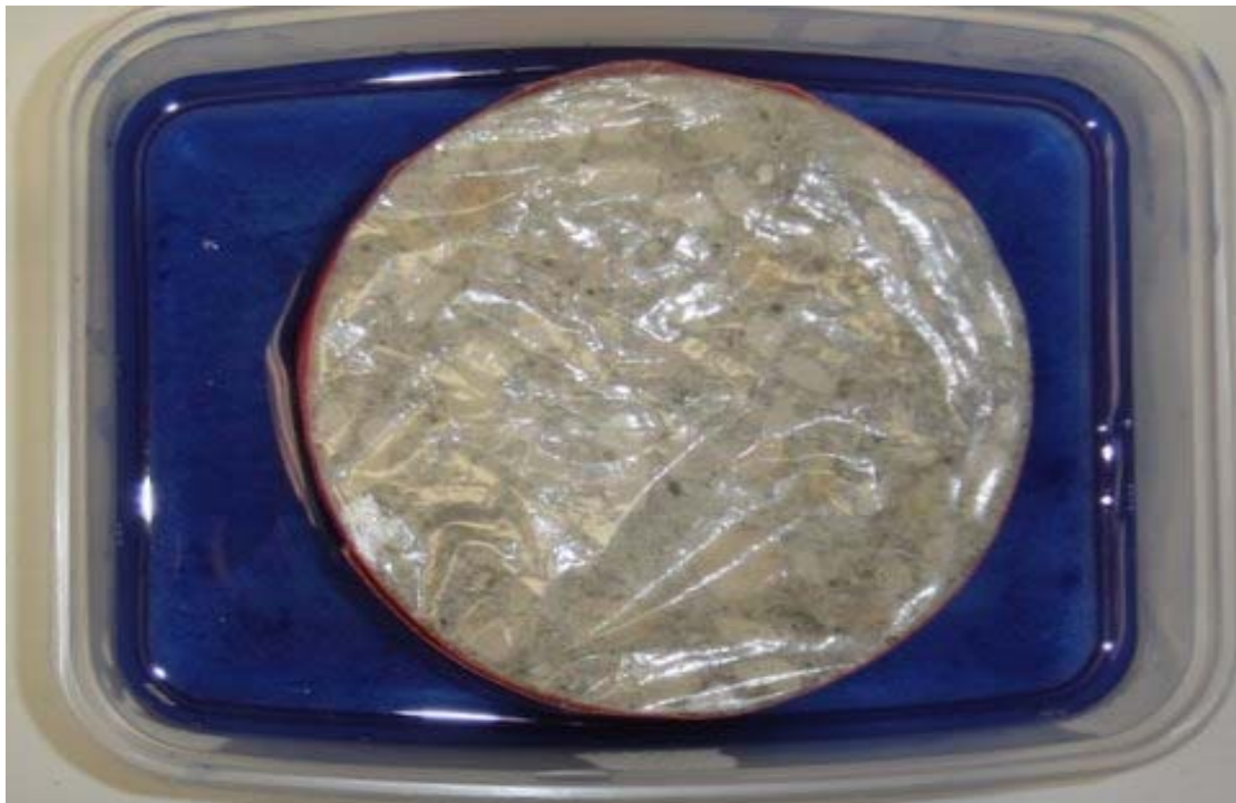
Photo (3): Lightweight concrete sample after one day's testing shows no trace of water on the top surface.
