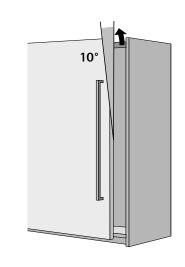
The door is pulled up and forwards at an angle with a defined
