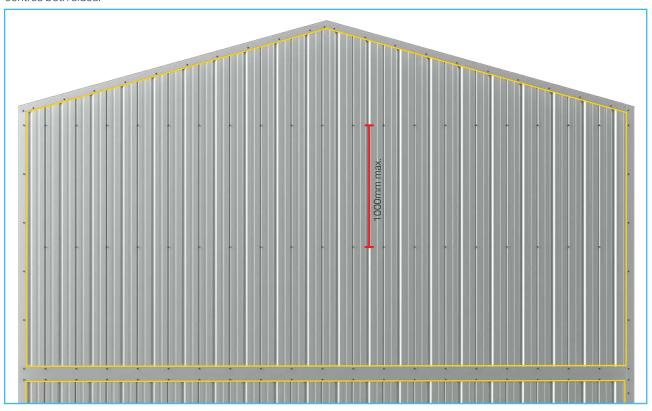
Ensure all C-track / panel junctions have been sealed with fire rated sealant.
