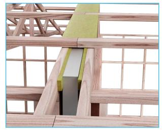
Install a KOROK® KIT flashing over the midwall joint fixed at 250mm centres top and bottom using 10x16mm Wafer Tek screws.
