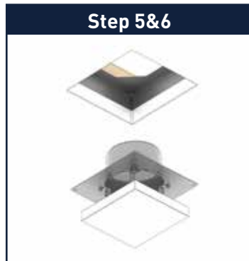
Centre tile installing
