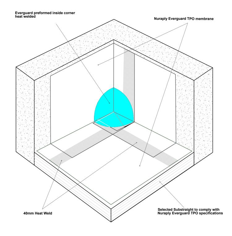
Everguard TPO field fabricated cut from non-reinforced membrane
