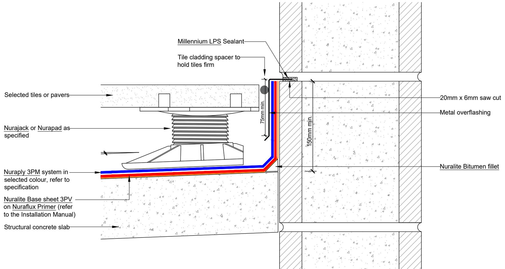
This drawing is indicative only and not for construction. This detail depicts Nuralite products and components for correct use as per the installation manual. All other elements are typical only - refer to the designer. Always refer to original colour details when printing.
