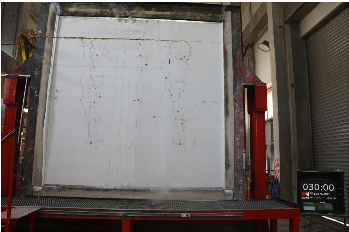
Photo 2: The Unexposed Face of the Specimen After a Duration of 30 Minutes
