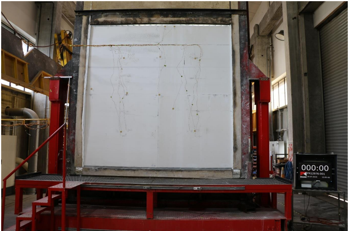
Photo 2: The Unexposed Face of the Specimen After a Duration of 30 Minutes
