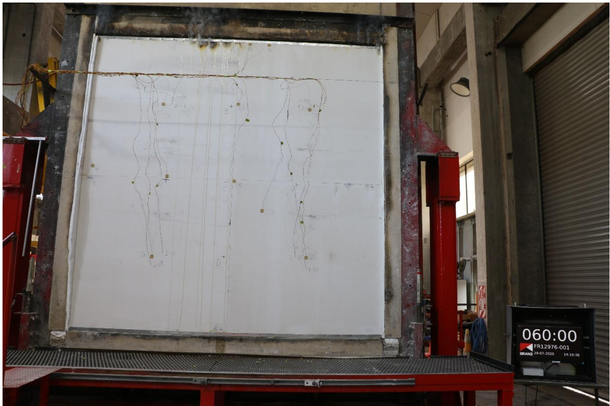
Photo 4: The Exposed Face of the Specimen Immediately After Testing
