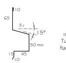
(Dimensions are indicative only in mm) Turn down end of head flashing to jamb flashing
