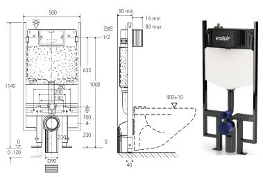
Max working pressure for all cisterns is 5 bar (500Kpa). Test pressure is 20 bar (2000Kpa) Please check wall hung pan set for correct installation height. Max weight 250kg.
