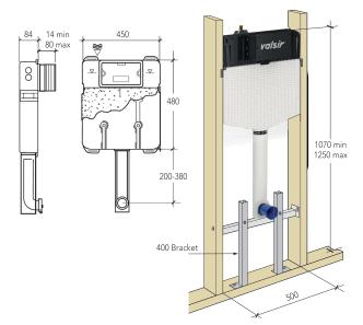
Max working pressure for all cisterns is 5 bar (500Kpa). Test pressure is 20 bar (2000Kpa) Please check wall hung pan set for correct installation height. Max weight 250kg.
