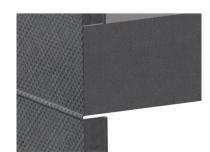
Figure 3. Compensation fold at expansion joints
