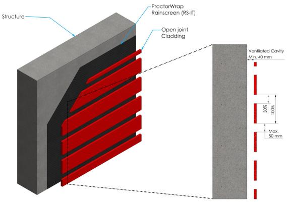
Figure 2. Allowable conditions for use with open joint rainscreen cladding
