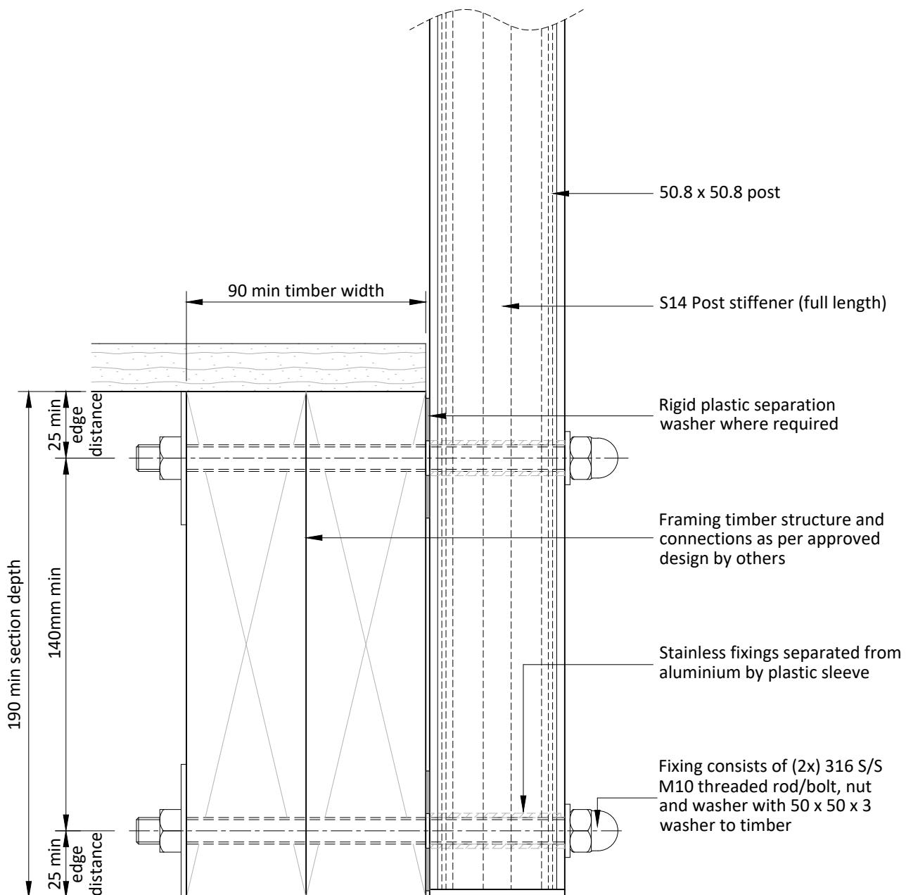
Leverage height max (distance from top of handrail to centreline of the upper fixing)
